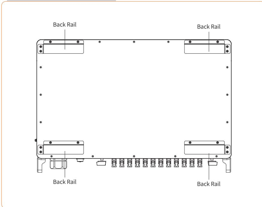
Figure 3-5 Inverter back view
